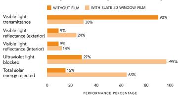
All performance results are based on the film installed on the inside surface of 1/8" (3mm), 1/4" (6mm), and 1/8"+1/8" (3mm+3mm) thick, clear glass.
